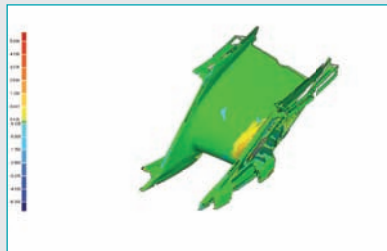
Scanned NGV using verification colour mapping comparing the actual scanned data back to the nominal CAD data
