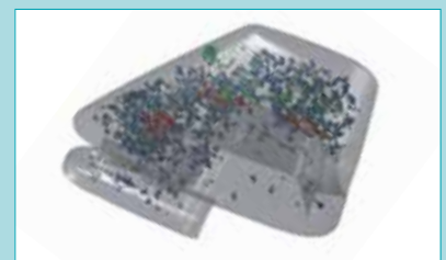
The 3D porosity analysis shows the size, distribution and position of the voids in the component
