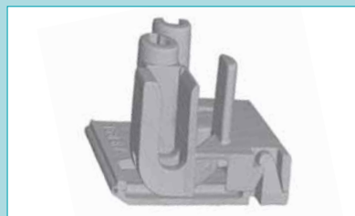
Virtual 3D section through the connector: the closing mechanism can be checked when it is closed.
