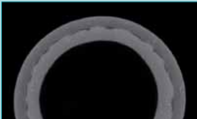
Transverse and longitudinal section through a hydraulic hose: the different rubber composition is revealed by grey tones. Inclusions in the material can be detected as bright points
