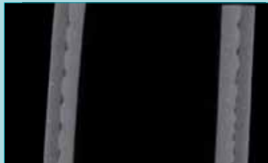
Transverse and longitudinal section through a hydraulic hose: the different rubber composition is revealed by grey tones. Inclusions in the material can be detected as bright points
