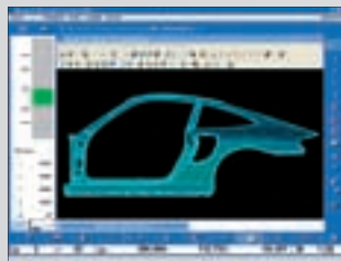
Measuring with direct comparison against CAD model data
