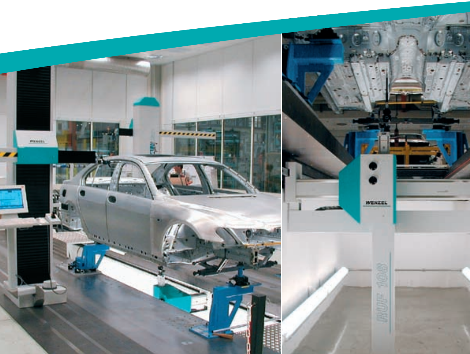
Both RA and RAplus series can be supplemented with the RUF allowing the workpieces to be measured from underneath.
