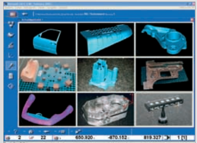
Automatic selection of part inspection programs with quick selection table
