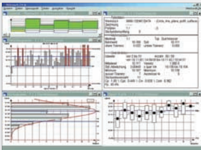
Configurable statistics: Overview, Trend diagram, SPC diagrams, Frequency distribution, Process capability etc.
