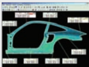
Graphic inspection report with CAD model and measured points
