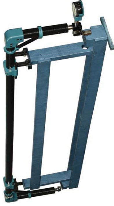
Special carbon fiber frame gage with master
